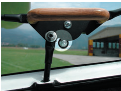
Incorrect - door not secured
