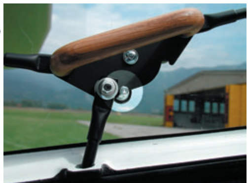
Correct - door secured
